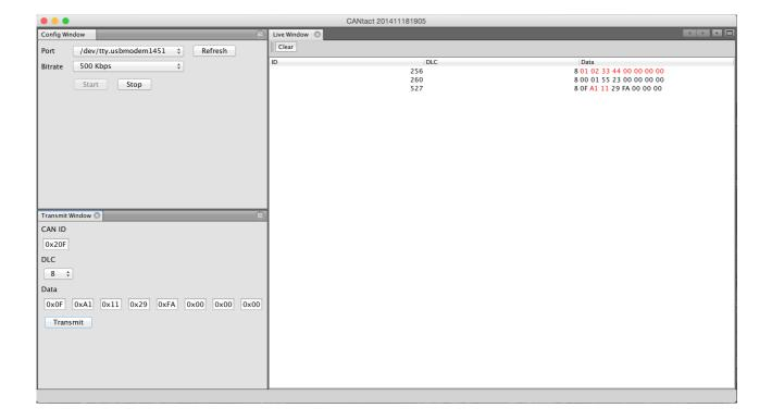
cantact-app (https://github.com/linklayer/cantact-app) is a Java program for viewing real-time CAN bus traffic and sending CAN packets. This tool connects directly to the virtual serial port of the CANable (or CANtact) device, and doesn't require any other drivers. Just download the latest release (https://github.com/linklayer/cantact-app/releases/download/v0.3.0-alpha/cantact-v0.3.0-alpha.zip), connect to your CANable, and traffic should show up shortly.
